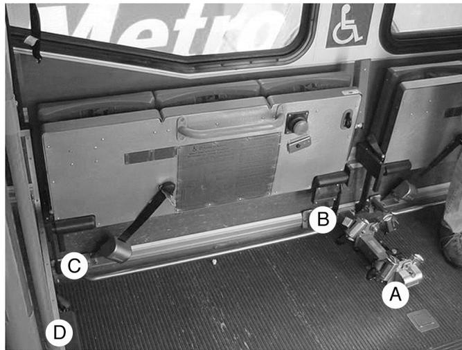
Figure 2. Wheelchair securement area on large transit bus (A=front aisle-side strap; B=front window-side strap; C=rear window-side strap; D=rear aisle-side strap (not shown))
