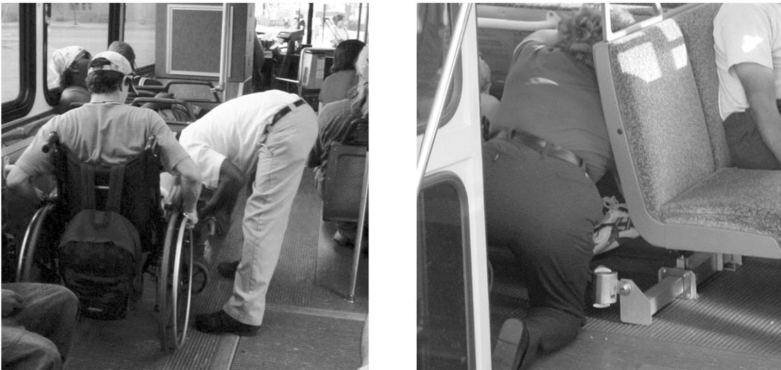
Figure 3. Operators securing a manual wheelchair into a transit bus.
